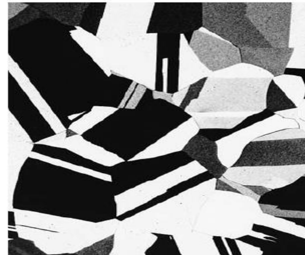
Figure 5.18 (a) Polished and etched grains as they might appear when viewed with an optical microscope. (b) Section taken through these grains showing how the etching characteristics and resulting surface texture vary from grain to grain because of differences in crystallographic orientation. (c) Photomicrograph of a polycrystalline brass specimen. 60 \times . (Photomicrograph courtesy of J. E. Burke)
